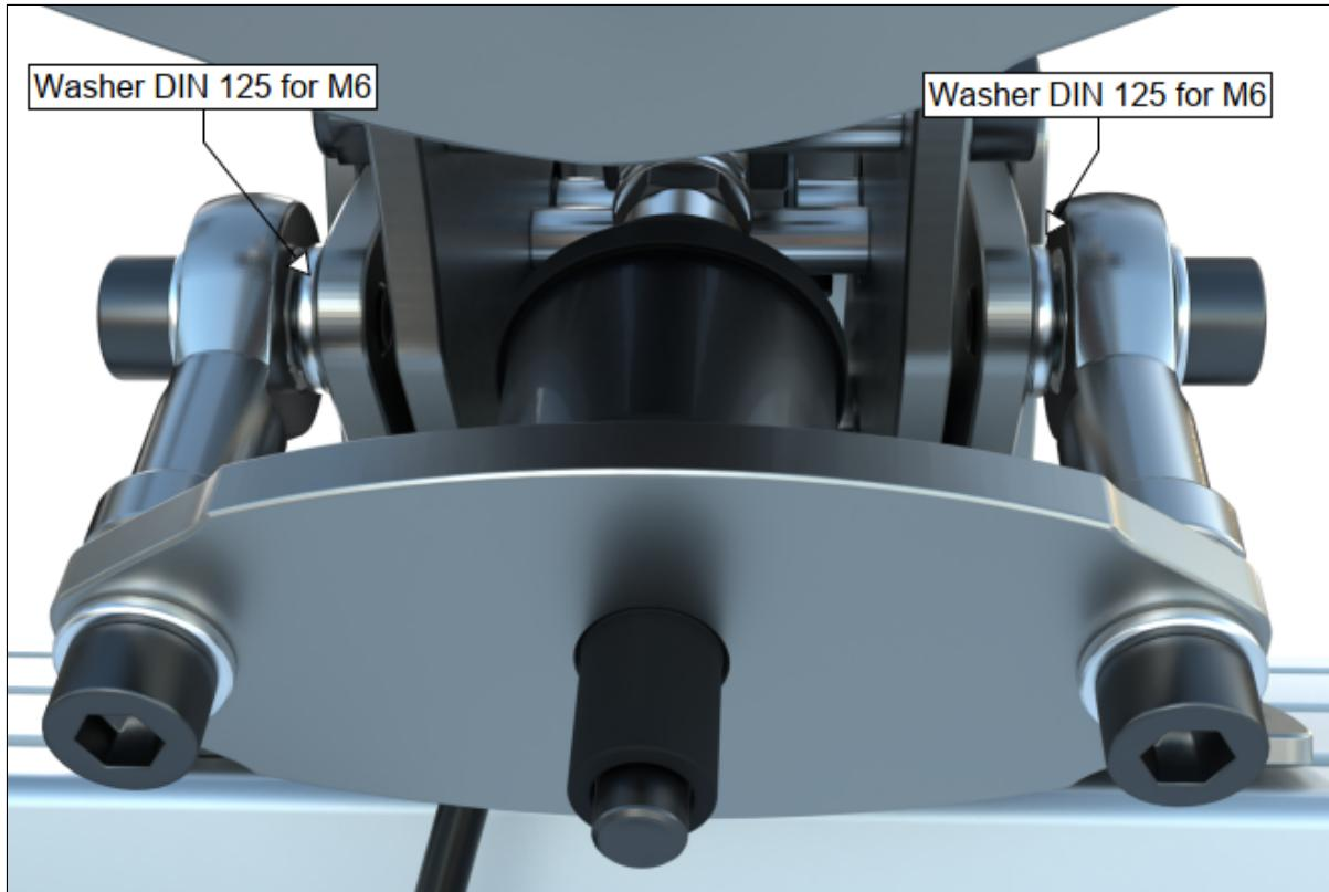
Install washers between the frame plate and the rod ends, see picture above. Tighten the M6-nut on the pedal arm end only so that the nyloc insert secures the connection, tightening more than that is unnecessary, see picture below.
