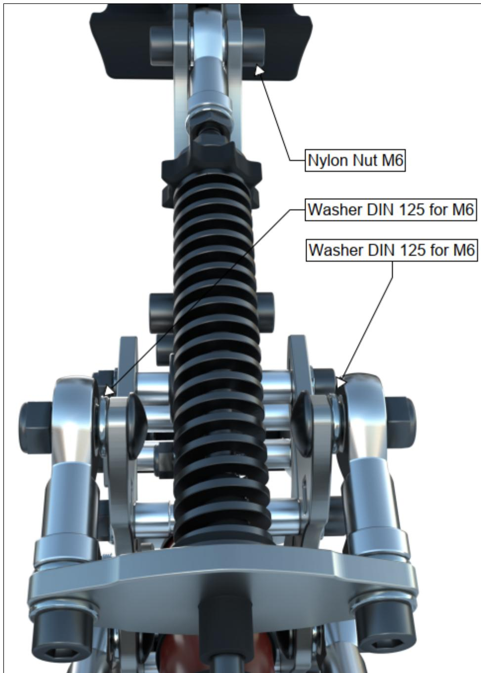
Install washers between the frame plate and the rod ends, see the picture above. Tighten the M6-nut on the pedal arm end only so that the nyloc insert secures the connection, tightening more than that is unnecessary.
